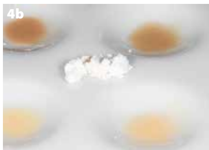
Fig. 4b: Addition of SPS-1 (Ivory White), SPS-2 (Melon Yellow) and some glaze powder.
